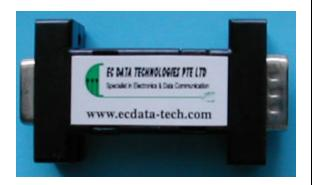
The ECD232TTL is designed to convert the RS-232 level signals into TTL/CMOS level signals. The unit allows you to connect a TTL device, such as the serial port on the micro-controller, to the serial port of the PC. The conversion circuit is housing inside the DB9 adaptor housing and the power is supplied from the micro-controller board.
