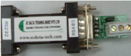
The ECD485nc provides excellent versatility in a compact package. Requiring no AC power or batteries for operation, the converter supports asynchronous RS-232 data rate up to 115200 bps over one unconditioned twisted pair in half duplex mode.
