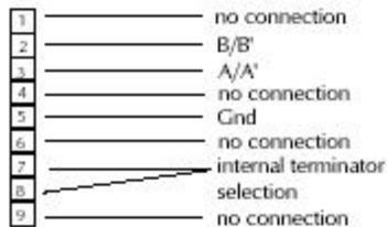
*Note: Short Pin7 & Pin8 to activate the internal terminator (120 Ohm)*
